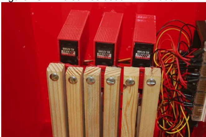
Figure 19. One servo motor controlling two pistons.
